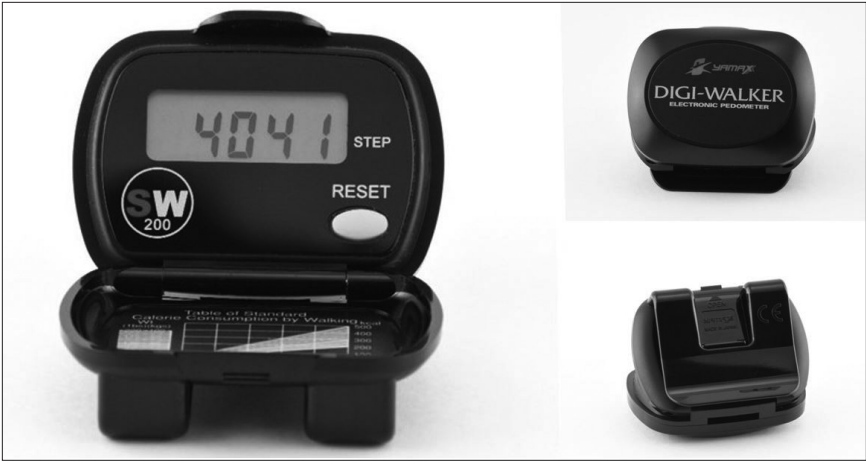
Figure 1. An open (left) and closed (upper-right corner) pedometer (Yamax SW200 Digi-walker) with a clamshell design and featuring a built-in clip (lower right corner). All images retrieved from www.yamax.co.uk . Reprinted with permission from the copyright holder.
